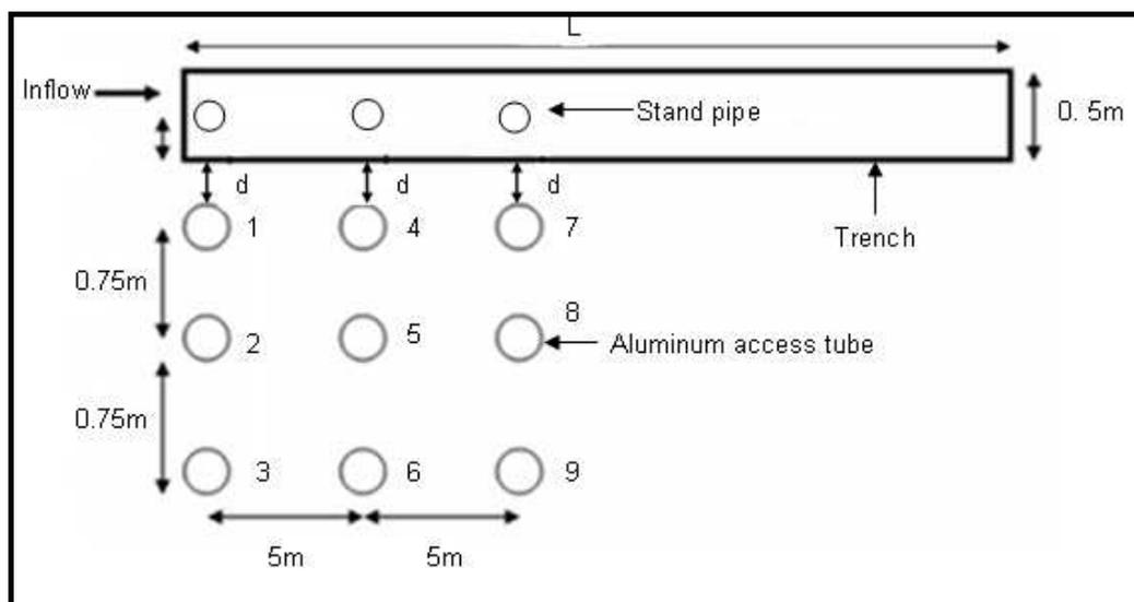
Figure 2: Plan view showing soil moisture and ponding level monitoring points relative to each study trench (not to scale).
