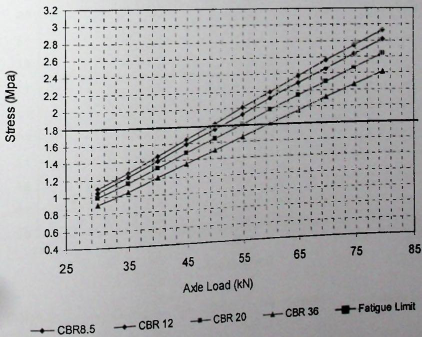
Figure 5.7: Loads vs. Stress relationship for a slab thickness of 125mm
