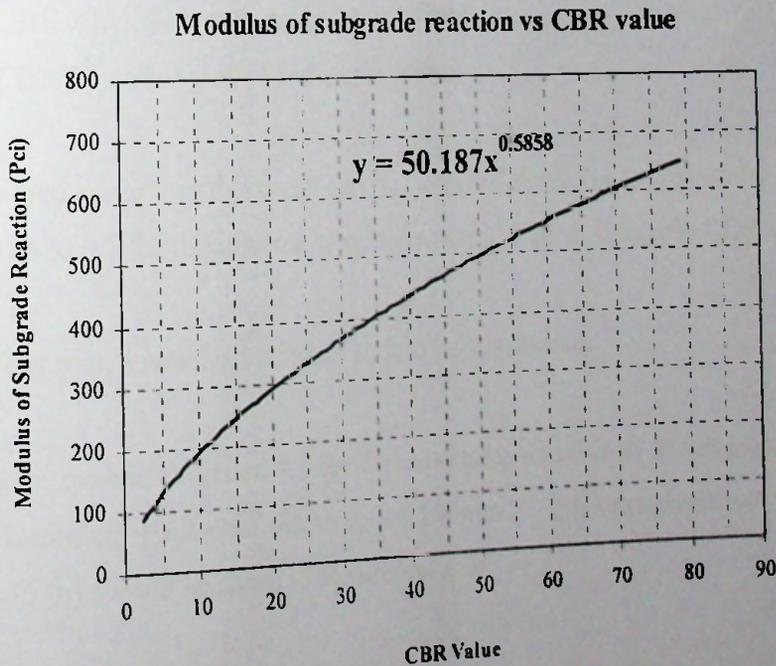
Figure 5.5: Modulus of subgrade reaction vs CBR value
