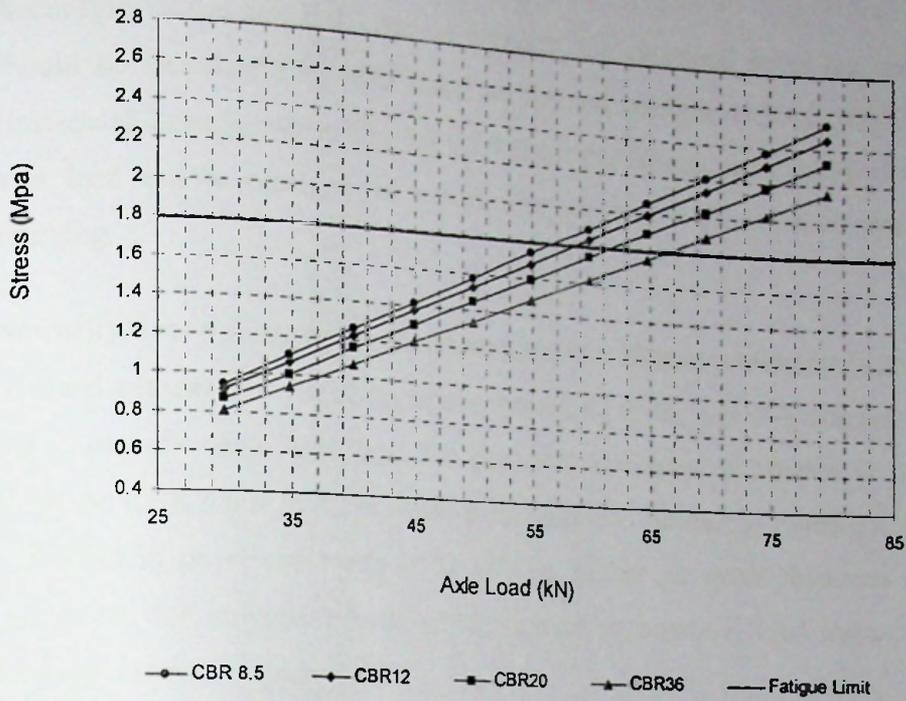
Figure 5.8: Loads vs. Stress relationship for a slab thickness of 137.5 mm
