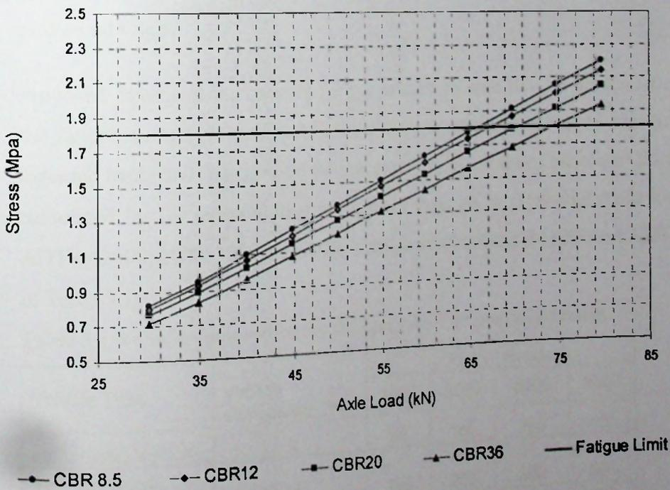
Figure 5.9: Loads vs. Stress relationship for a slab thickness of 150mm
