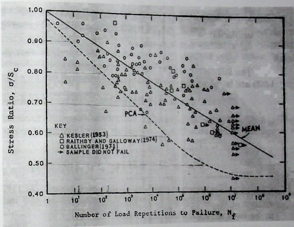
Figure 5.10: Fatigue tests results on concrete
