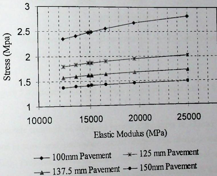
Figure 5.3: Stress variation for different Elastic Modulus for 52 kN axle load
