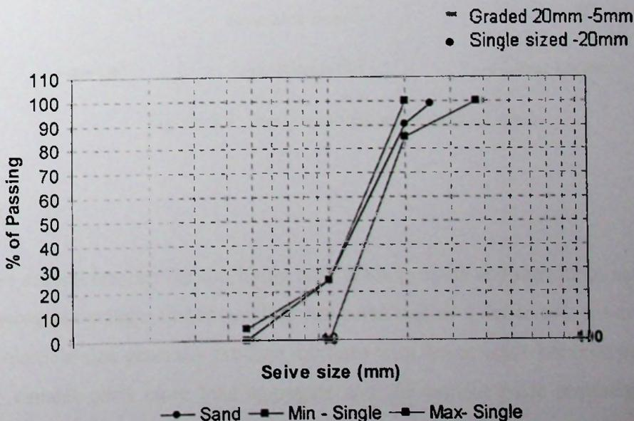
Figure 4.2: Sieve analysis test result of RCM (Coarse Fraction Gradation)
