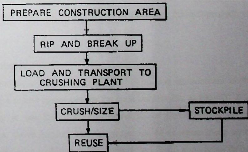
Figure 2.5: Recycling Portland cement Concrete flow chart
