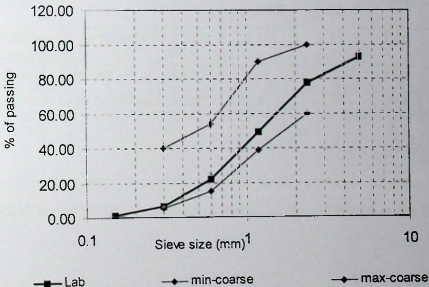
Figure 4.3: Sieve analysis test result of sand
