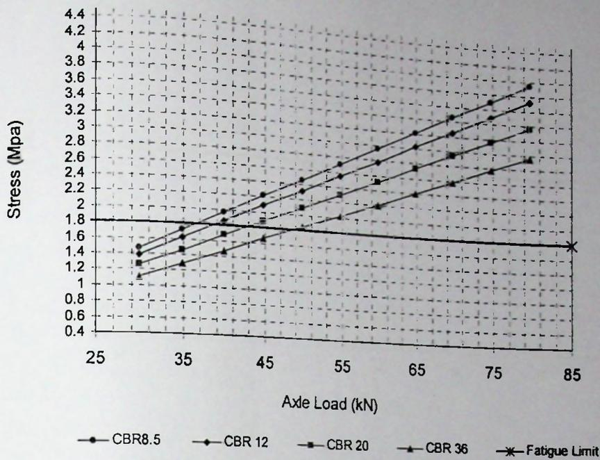
Figure 5.6: Loads vs. Stress relationship for a slab thickness of 100mm
