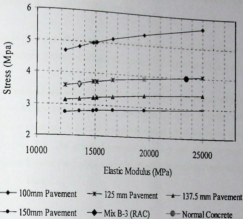
Figure 5.4: Required flexural strength to limit the stress ratio to 0.5
