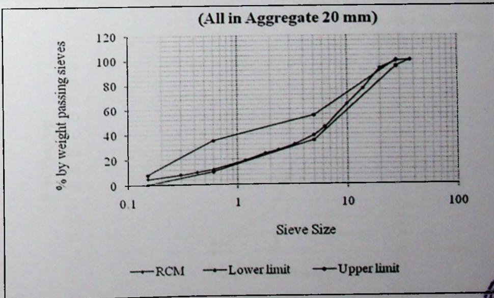
Figure 4.1 Sieve analysis test result of RCM (Overall Gradation)
