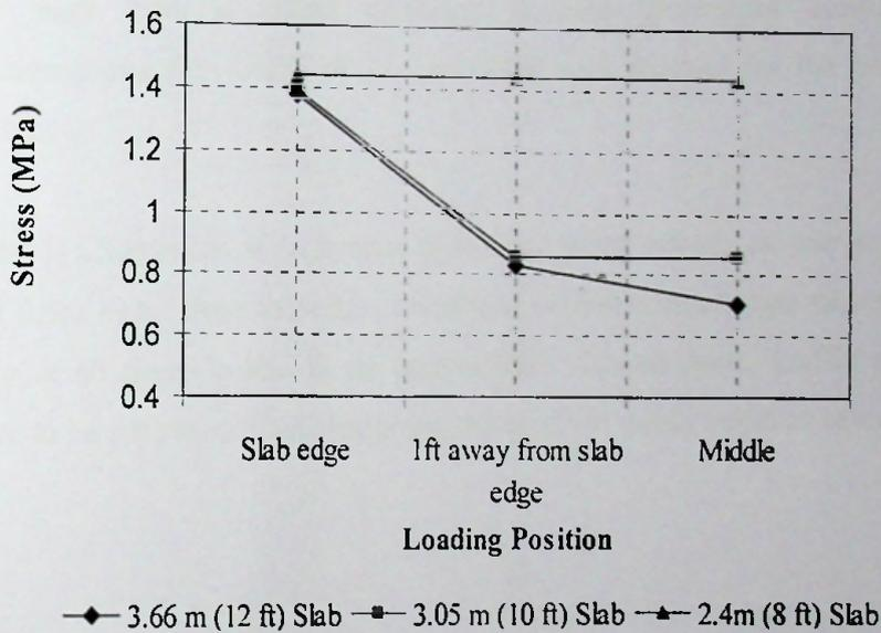
Figure 5.1: Stress Variation according to Slab width
