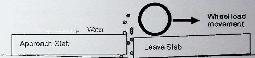
Figure 2.4: Pumping action failure of the slab
