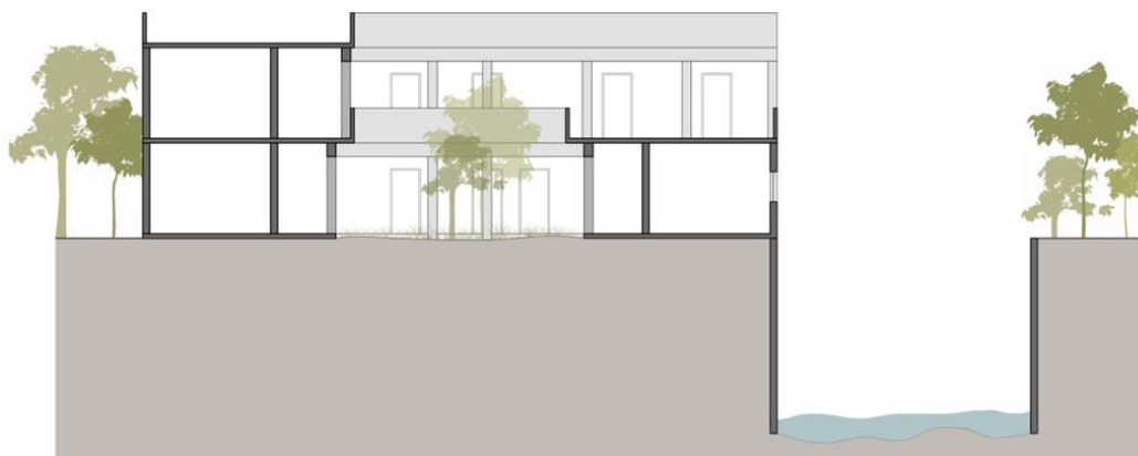
Figure 20: Section: No windows in classrooms on east façade; west façade shares its boundary wall with the Baoli Source: author
