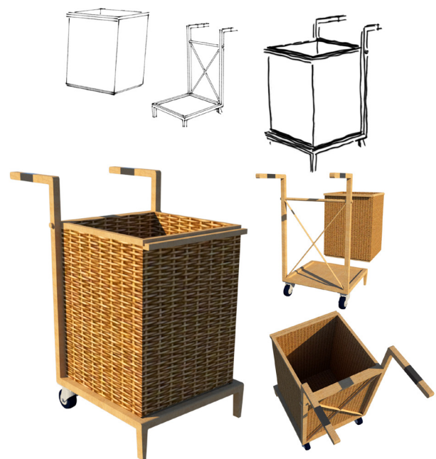
Figure 3: Design Solution - Hump Storage Which Combines Both Harvesting and Storing Process
