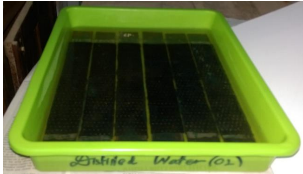
Figure 8.2: Samples immersed in distilled water at room temperature (25°C-30°C)
