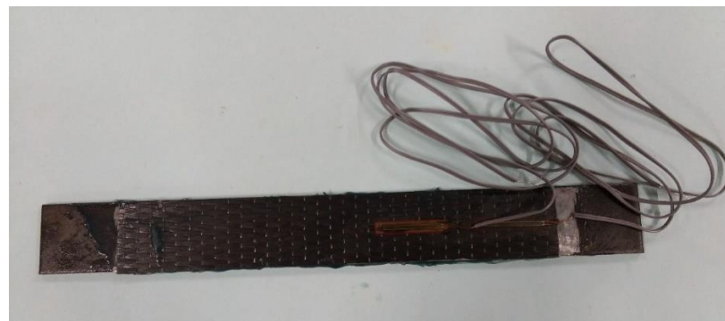
Figure 5.7: Prepared test specimen of a double strap joint
