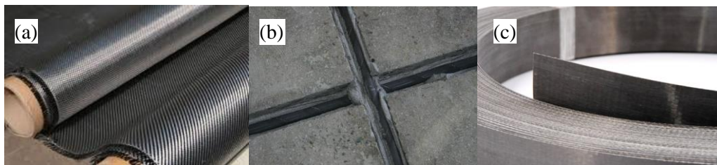
Figure 2.1: Different forms of CFRP (a) Fabric (b) Rods (c) Strips
