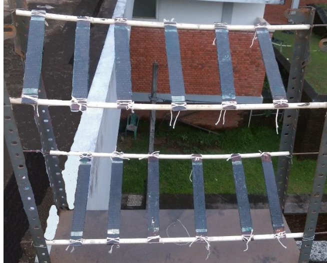
Figure 8.5: Samples exposed to tropical environmental condition
