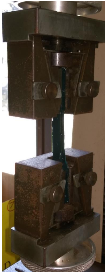
Figure 3.8 (b): Test setup of an adhesive coupon
