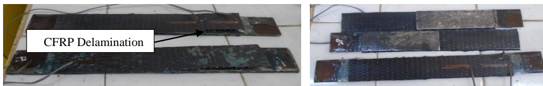
Figure 6.7: Failure modes observed for the specimens
