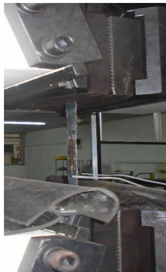
Figure 3.3: Test setup of a CFRP test coupon specimen
