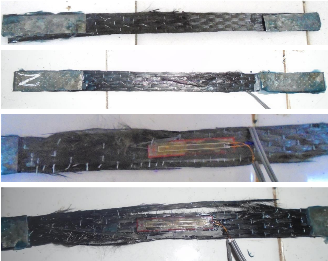
Figure 3.4: Failure mode (Edge Delamination in the Middle Gauge area) of CFRP coupon test specimens
