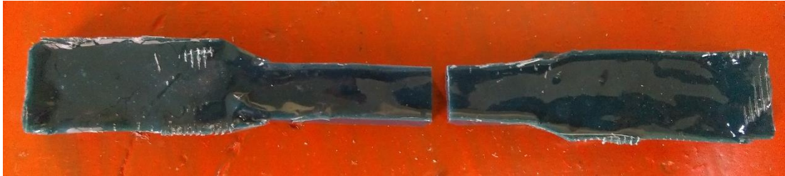
Figure 3.9: The failure mode of an adhesive coupon
