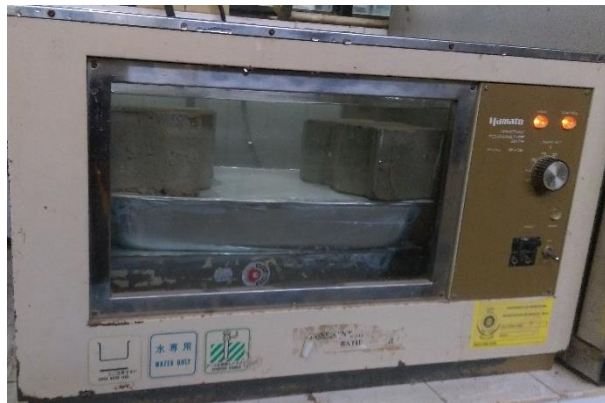
Figure 8.3: Samples immersed in distilled water at 40°C
