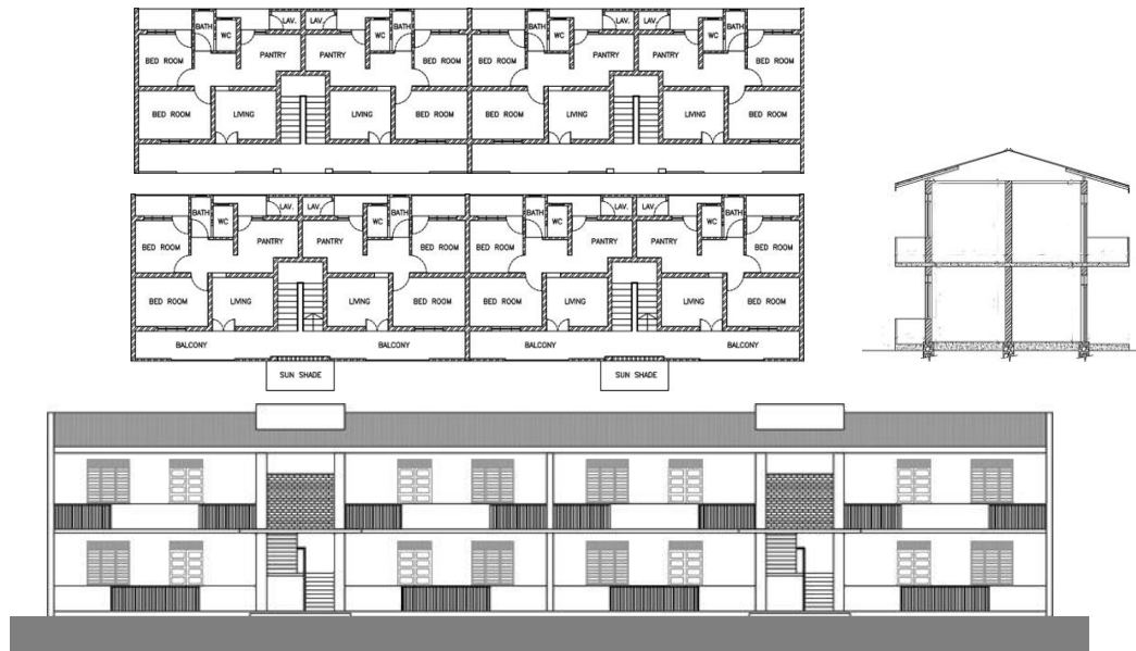
Figure 4.29: Two storied block type with two-bedroom housing type option; Ground and Upper floor Plans, Elevation, Section
