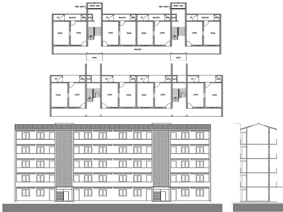
Figure 4.30: Five storied block type with single bedroom housing type option; Ground and Upper floor Plans, Elevation, Section Source: National Housing Development Authority, 2018
