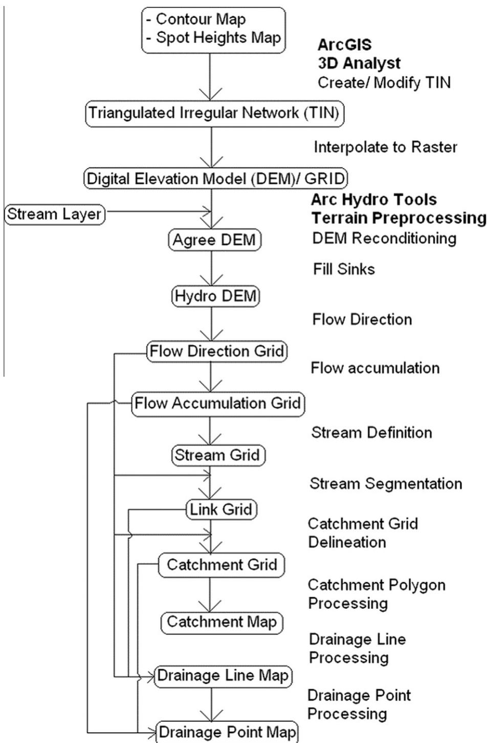
**Figure 4** Flow sheet of the hydrological analysis of the Suriyawewa DS area, Hambantota District, Sri Lanka.
