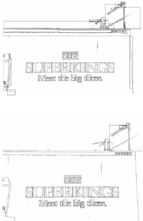
Figure 2: Contour identification. Top: all identified contours, Bottom: only possible letters
