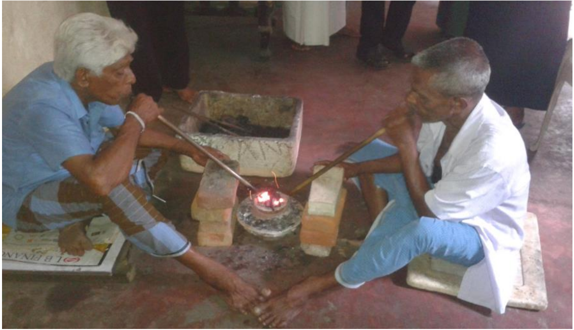
Figure 2: Operation of the Blow Pipe with two people
