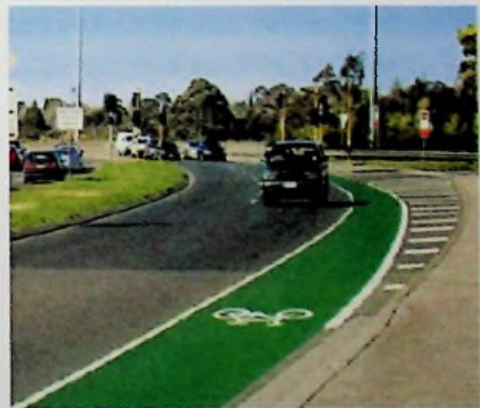
Figure 2.13: Road marking and Colour surface demarcated for cycle users
