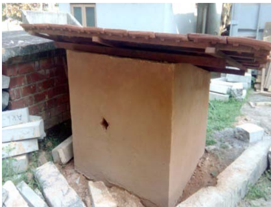
Figure 1: Model with mud concrete panels
