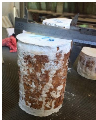
Figure 5, Applied capping on both side of MC sample
