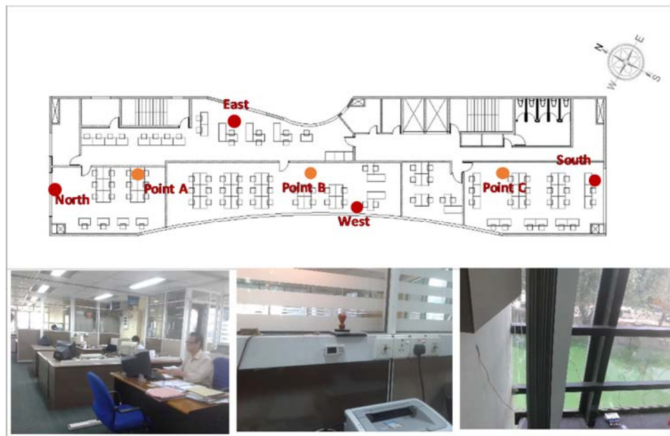
Figure 30: Instrumentation arrangement of the apparatus on the floor plan
