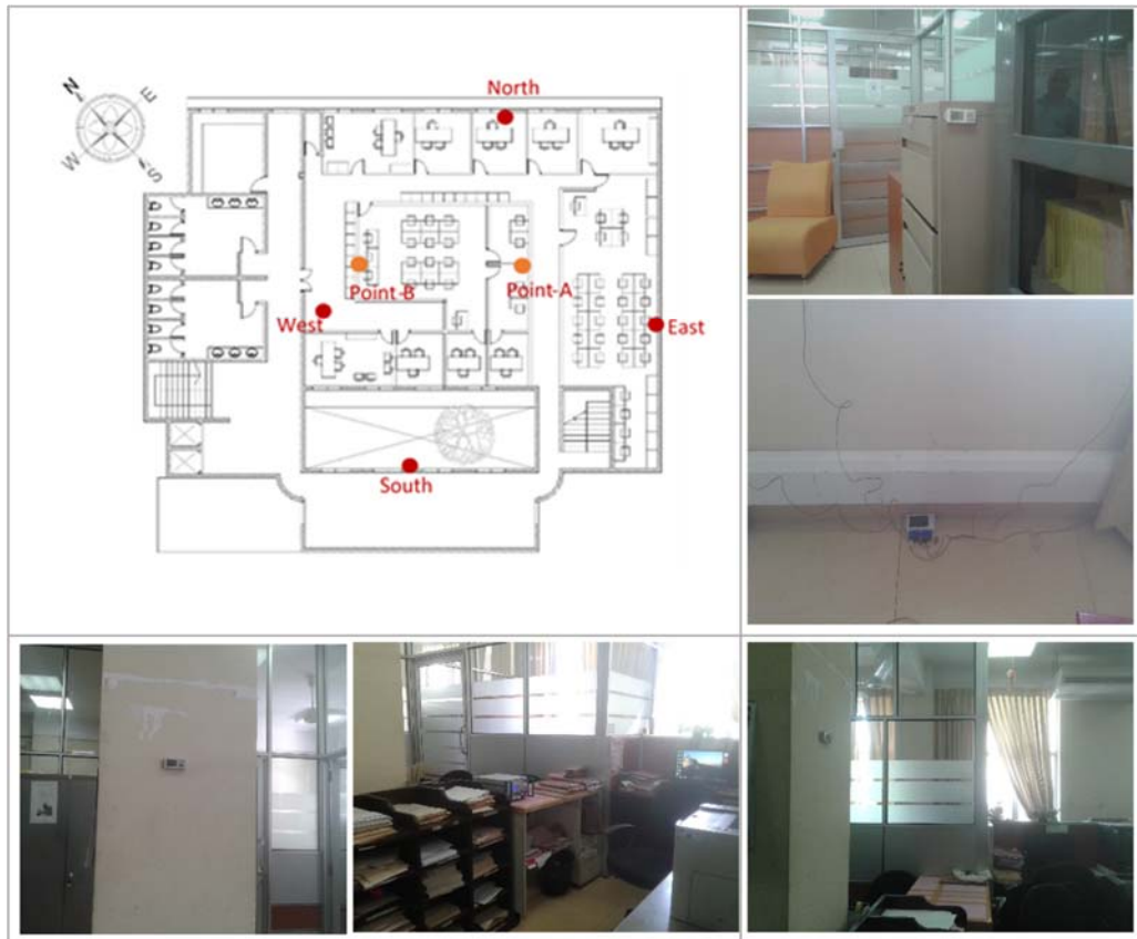
Figure 12: Instrumentation of data loggers in the floor plan
