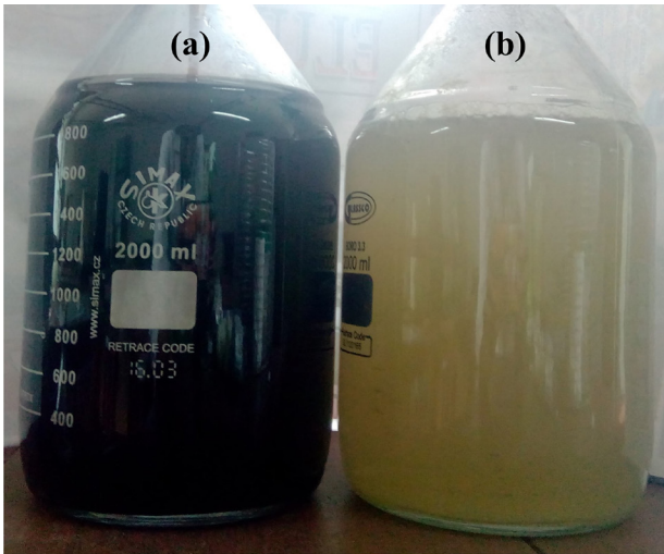
Figure 2: a). Influent (50ppm synthetic dye mixture containing medium), b). Treated water obtained from continuous FBBR
