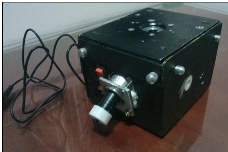
Fig 4.9: Box-shaped arrangement of the designed lubrication oil analyzer
