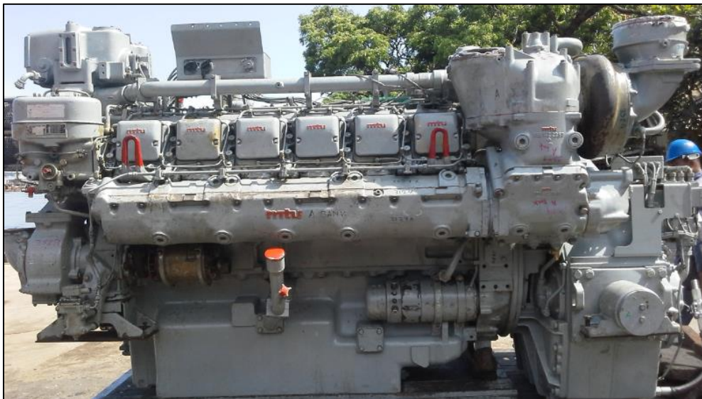
Fig 3.5: Real picture of a MTU 12V 396 TE 94 engine
