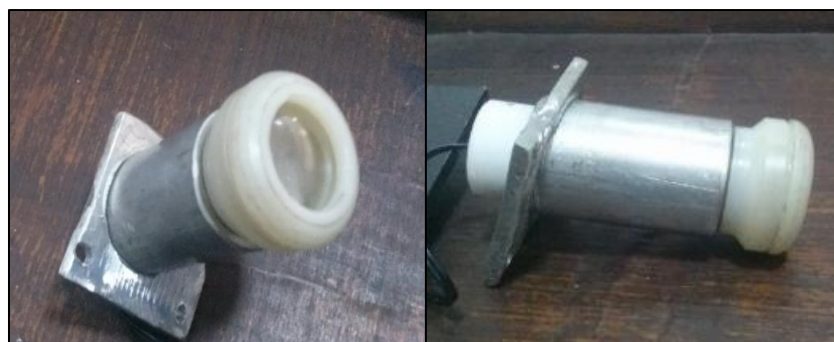
Fig 4.7: Arrangement of the light beam adjusting mechanism
