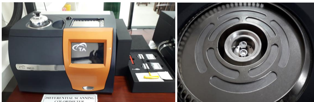
Figure 3.2: DSC analyzer placement of specimen
