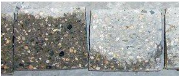
Figure 10: Water absorption by concrete
