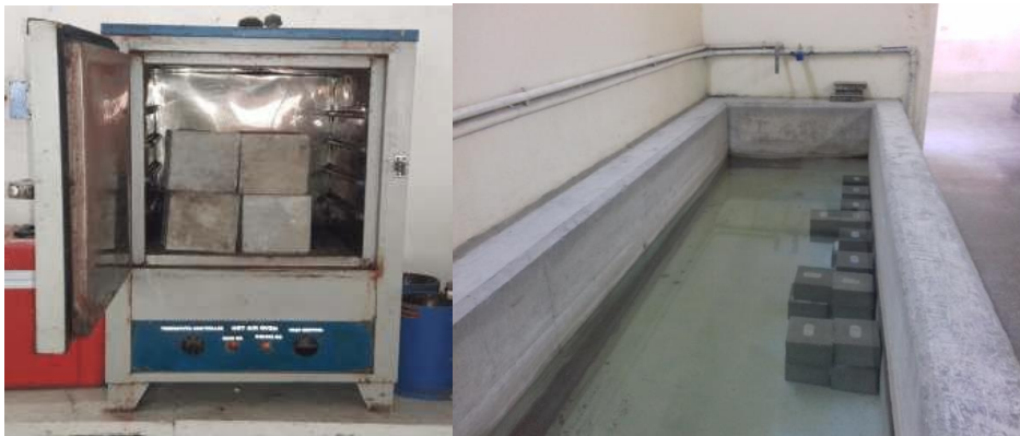
Figure 14: Shows the experimental setup of the water absorption test
