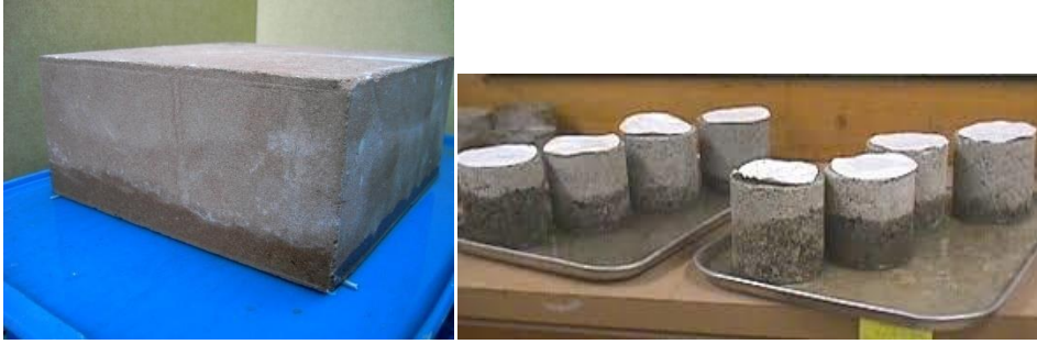
Figure 9: Demonstration of the capillary rise of hardened concrete
