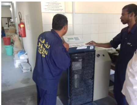
Figure 20: Shows the experimental setup of the cube crushing strength test
