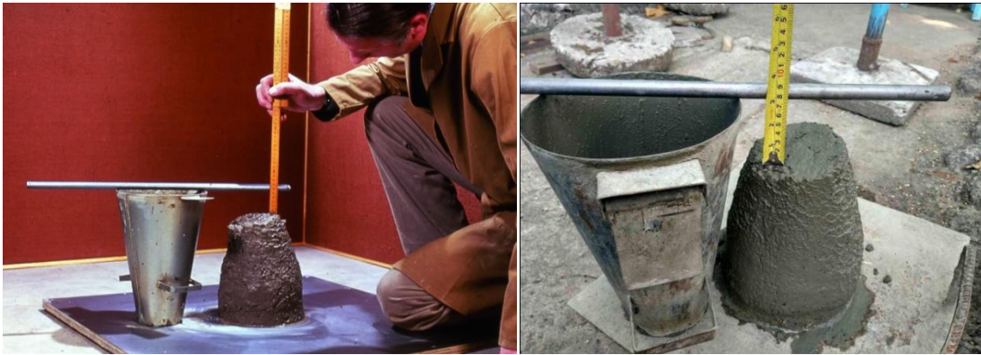
Figure 12: Measuring of Slump Height
