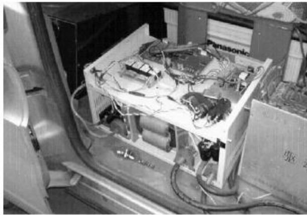
Figure 2.2.1.2 Energy management and control of electric vehicles, using a hybrid power source in regenerative braking operation hardware structure[1]
