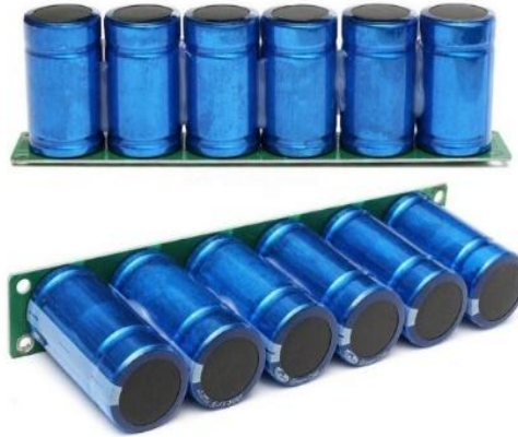
Figure 4.1.3.2 Super capacitor bank[11]
