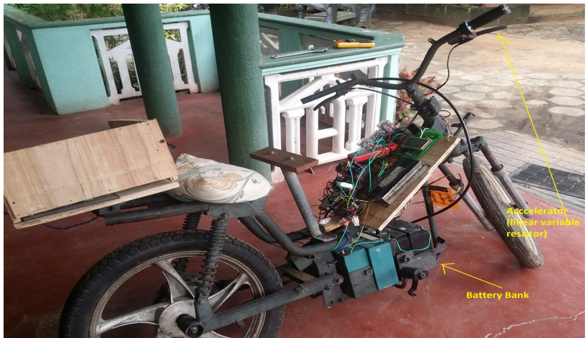
Figure 4.2.2 Side view of the complete system
