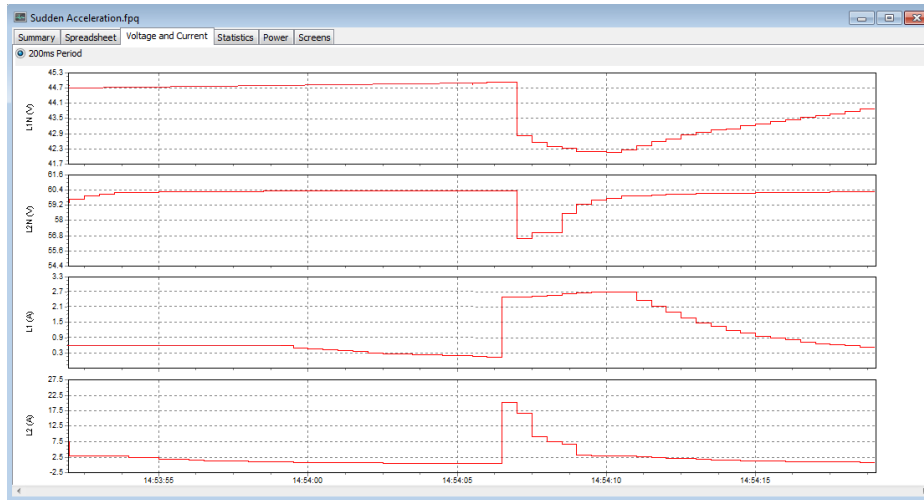
Figure 5.1.1.1 Sudden acceleration test result (no-load)-with super capacitor array
