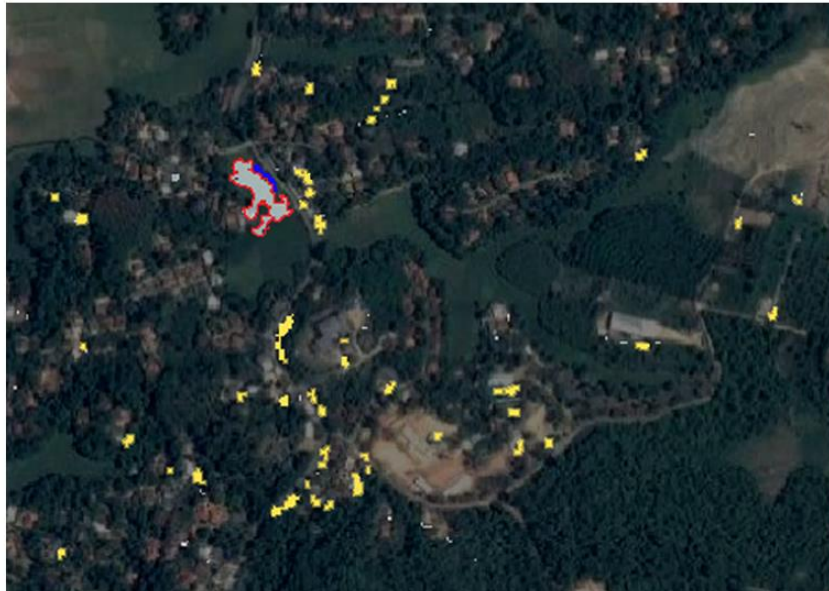
Figure 4.8 Identified damaged regions by the SVM model. Area covering true positive results is outlined in red. False positive results are colored in yellow. False negative results are colored in blue.
