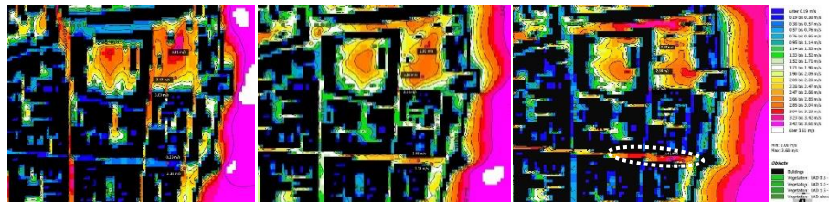
Figure 6: Site B - Wind velocity at 1.5m - S, SW, and W (from left to right)
