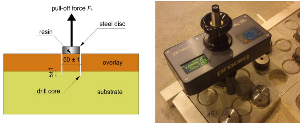
Figure 3.8: The scheme of the pull-off method (a) a view of the testing device (b).
