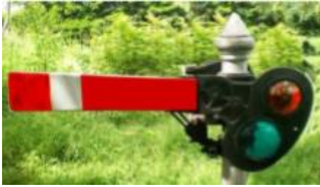
Figure 2.2: Semaphore arms in mechanical signaling
