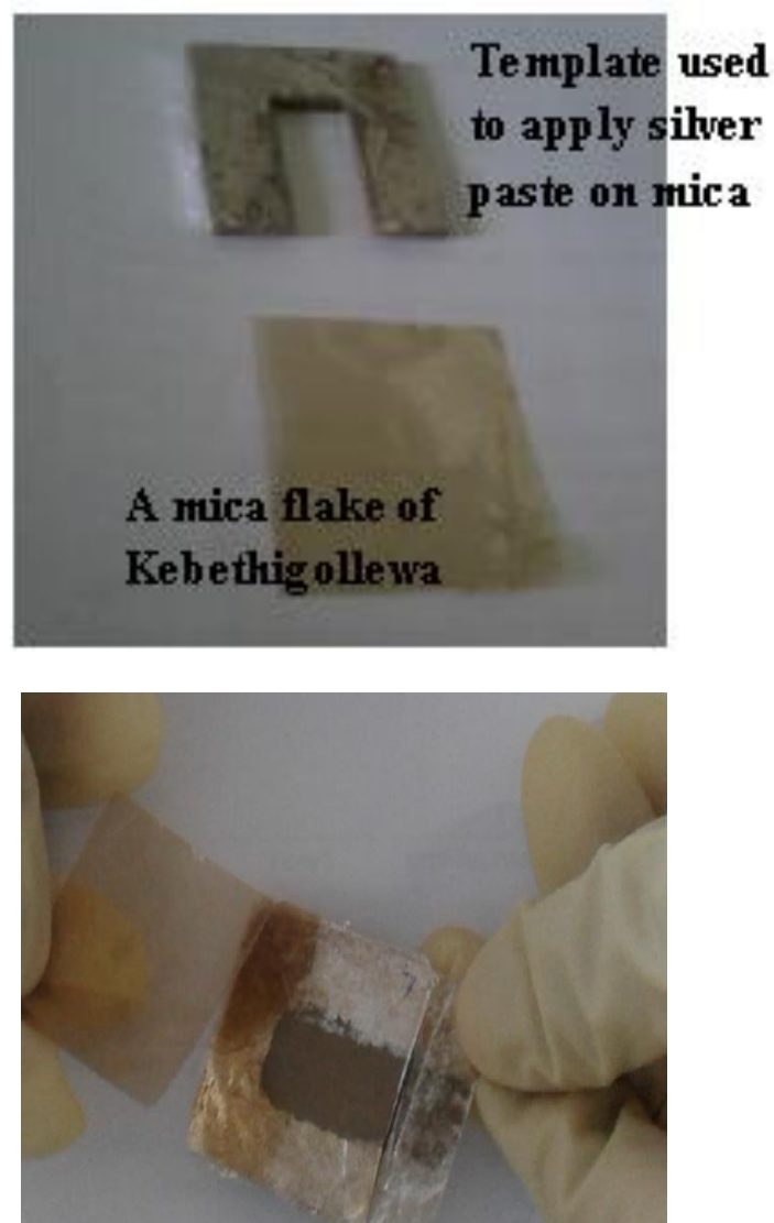
Figure 3.5: Application of silver paste on mica flakes
