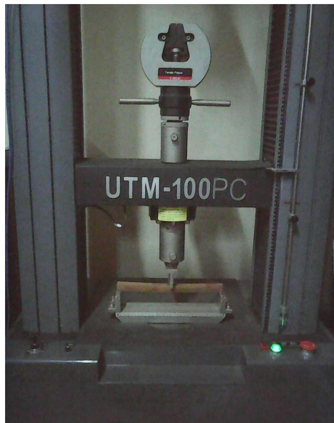
Figure 4.7 - Three point bending test through universal testing machine (Original in colour)
