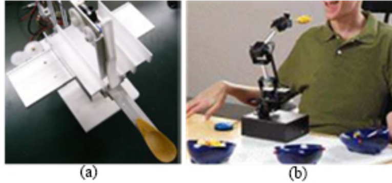
Figure 2.3: Foods storing methods. (a) The foods tray with tracks [17]. (b) Quadrant platform used in meal buddy [5].
