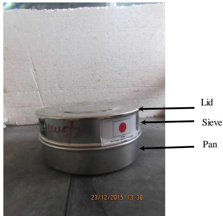
Figure 3.2: Dry sieving of CFA
