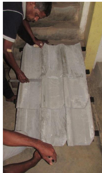
(d) Assessment of shape of overlapping ends
