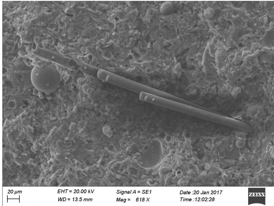
Figure 4.9: Fracture surface of the AR glass fibre reinforced fly ash-cement composite
