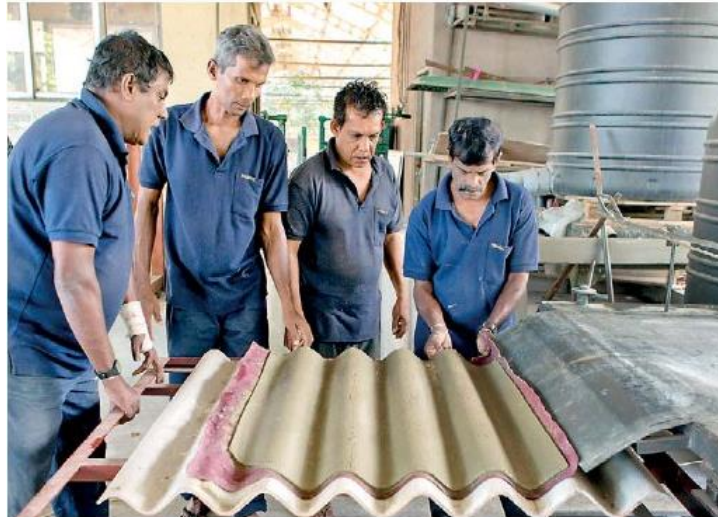
Figure 2.2: Manufacturing of MCR sheets at NERD Centre, Sri Lanka, J.A.C Chrishanthi et al [7]
