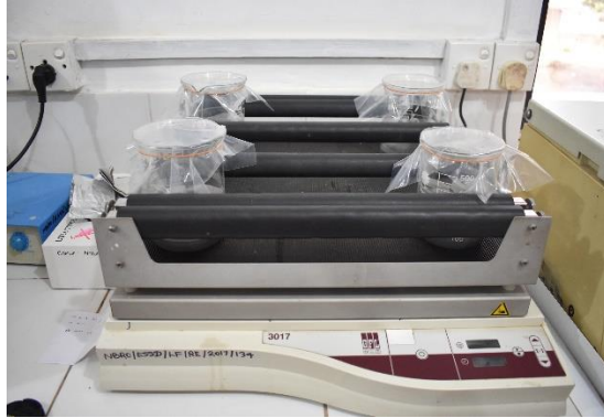
(a) Sealed beakers consist of CFA in acetone solution are being shaken in
