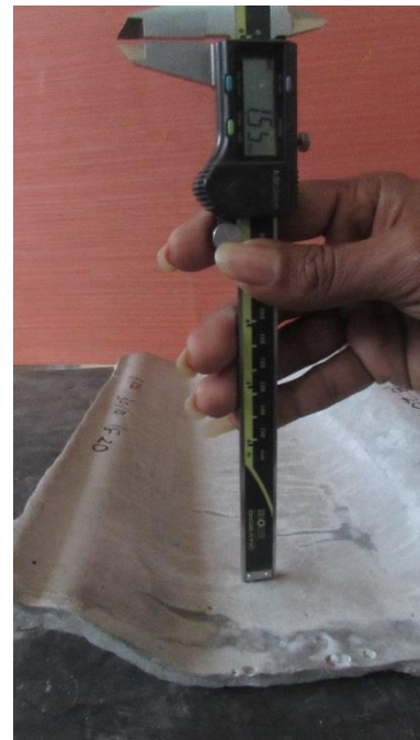
(c) Pore and crack test
