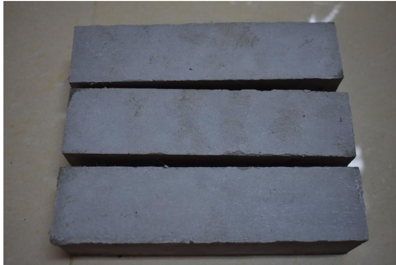
Figure 4.5: Coal fly ash-cement mortar prisms
