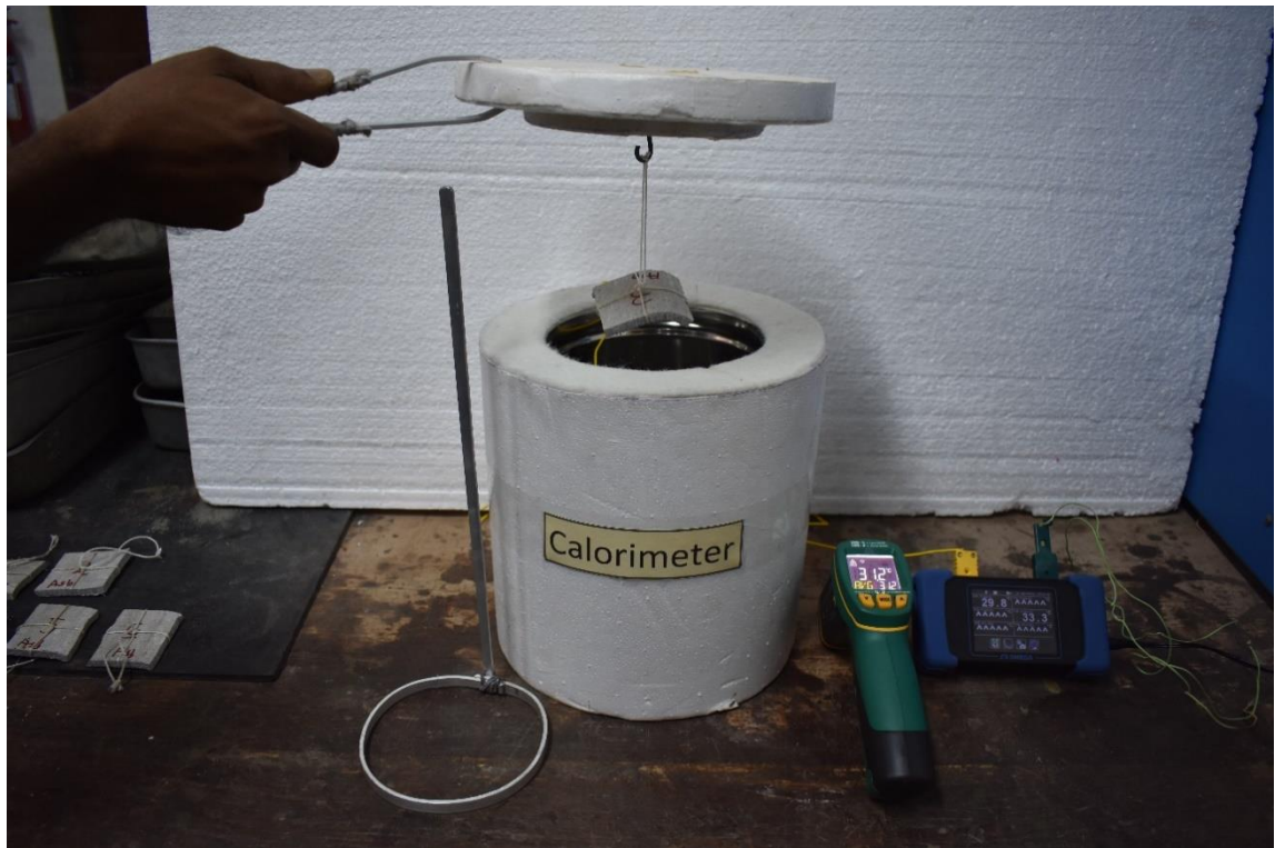
Figure 3.10: Experimental set up of the calorimeter
