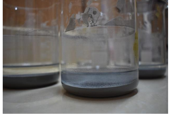
(b) After shaking, allowing CFA to settle for 16 hours
