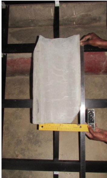
(a) Determination of hanging length and squariness
