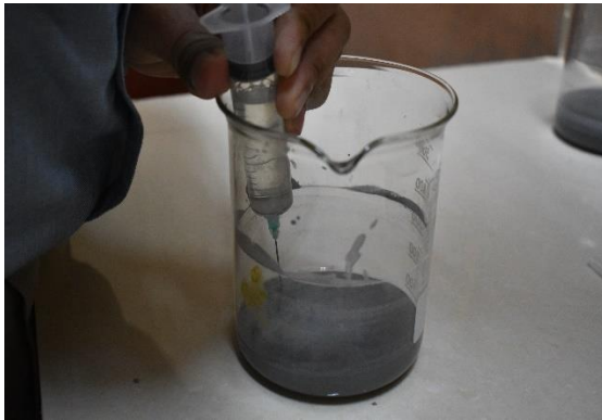
(c) Acetone is siphoned by a syringe
