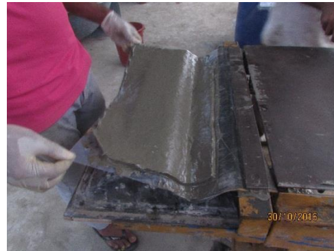
(d) Green mix is carefully taking onto the mould
