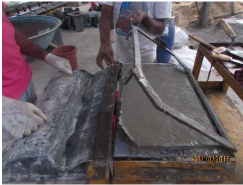
(c) Removal of frame once the levelling is done
