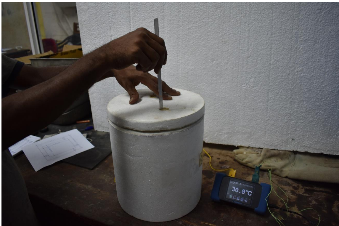
Figure 3.11: Continuous stirring until the temperature of water becomes equilibrium which is monitored by a data logger
