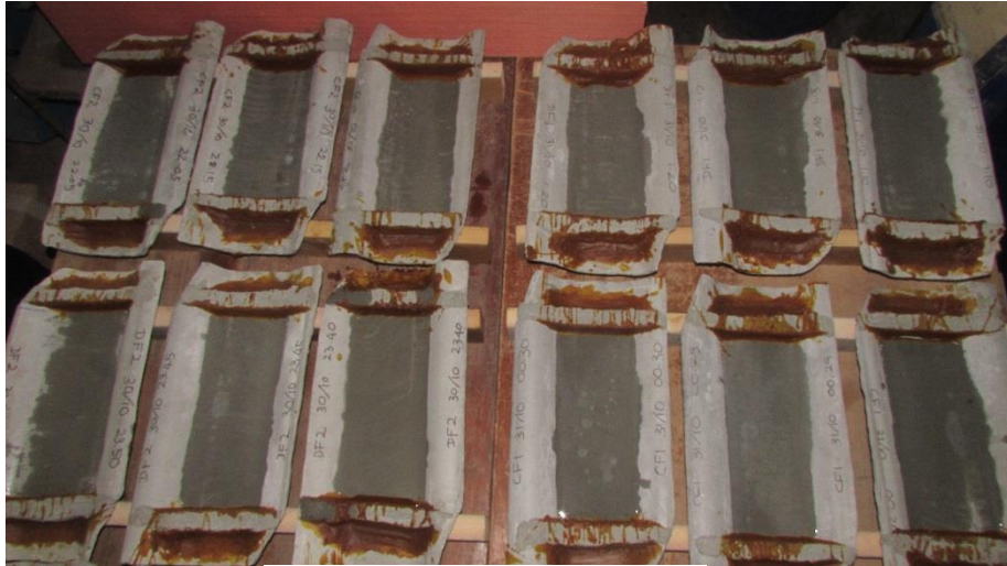
(a) Impermeability test
