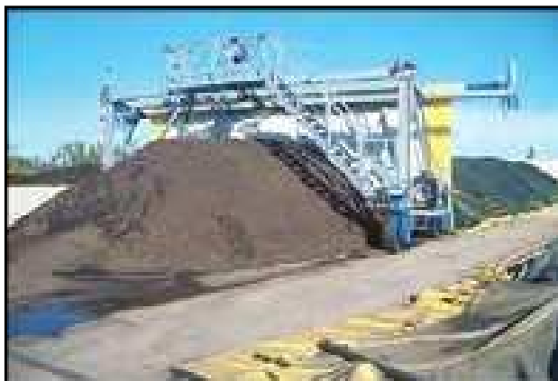
Figure.2.51: Covered, positively aerated composting system [17]
