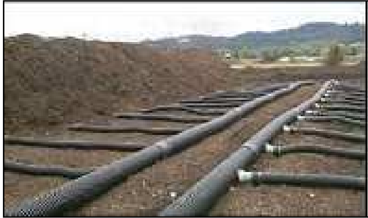
Figure.2.45: Typical passively aerated windrow system [17]
