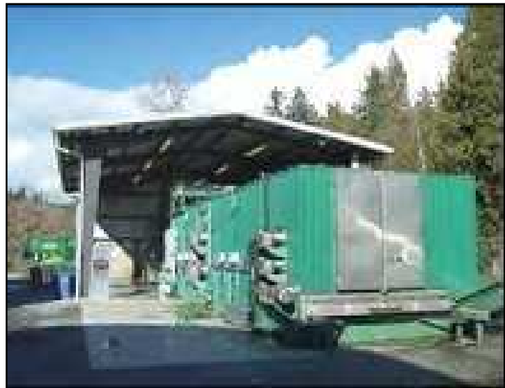
Figure.2.58: Agitated container composting system installed at a University Campus[17]
