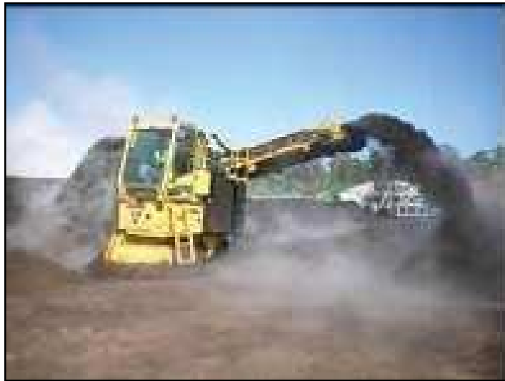
Figure.2.42: A self-propelled windrow turner used for turned mass bed Composting [17]
