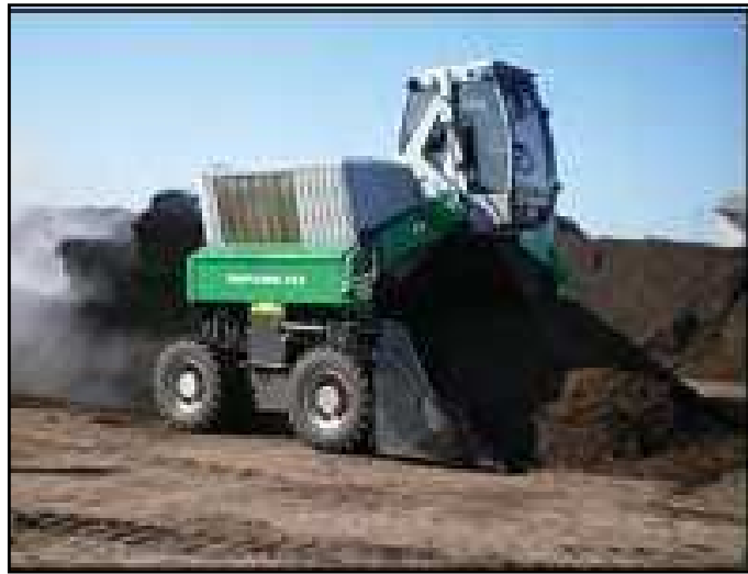
Figure.2.40: Straddle-style windrow turner [17]
