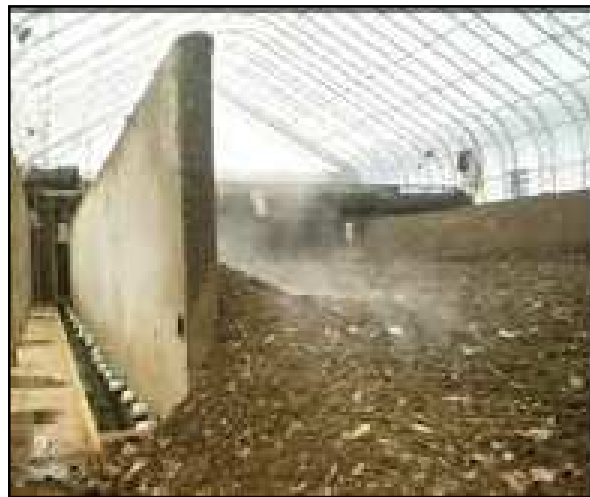
Figure.2.61: Agitated bed system viewed from discharge end of bay [17]
