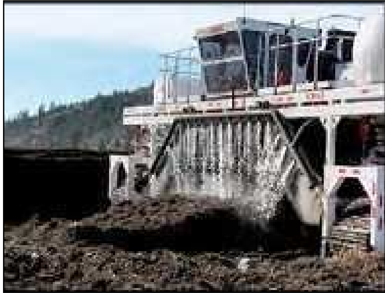
Figure.2.35: Water is best added to windrows when they are being turned [17]
