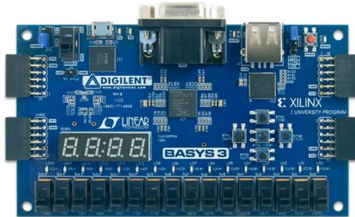
Figure 2-17 Basys 3 Artix-7 FPGA Trainer Board
