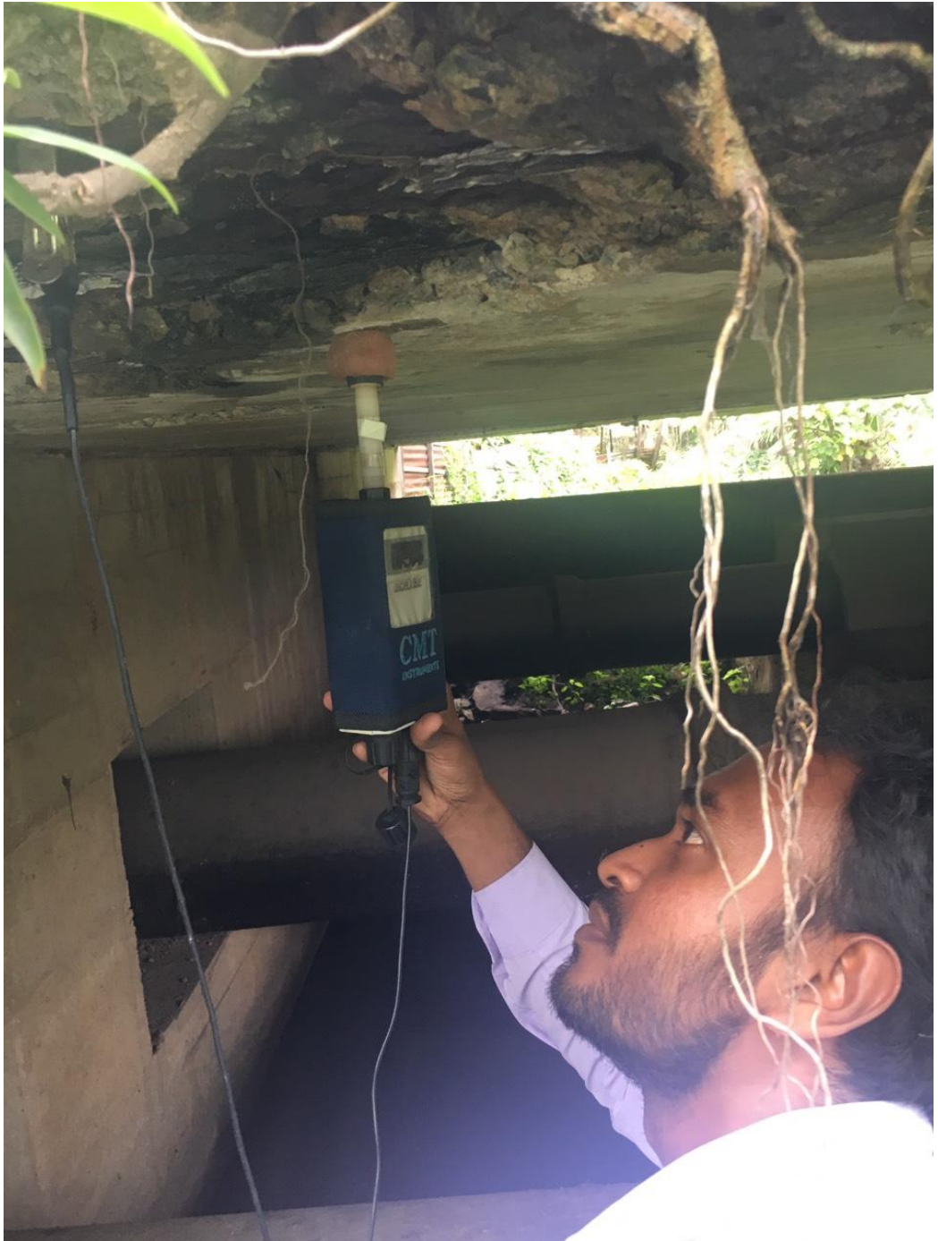
Figure 3-25 : Taking readings with half cell potential on an old bridge deck
