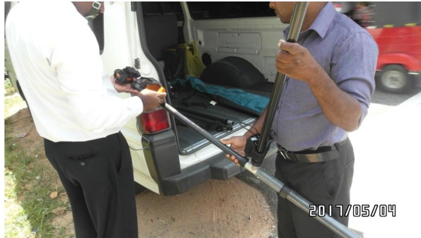
Figure 3-5 : Assemblage of pole camera during field inspections
