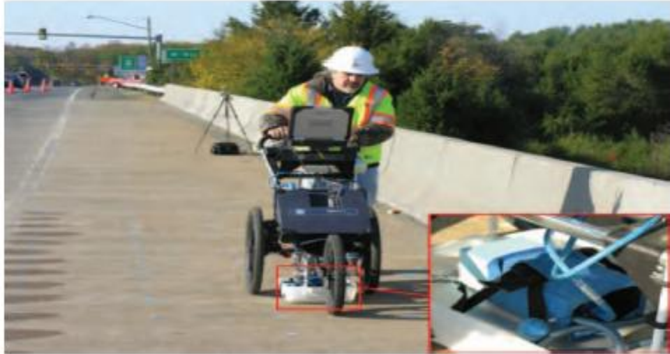
Figure 2-10: Bridge deck survey using GPR [17]
