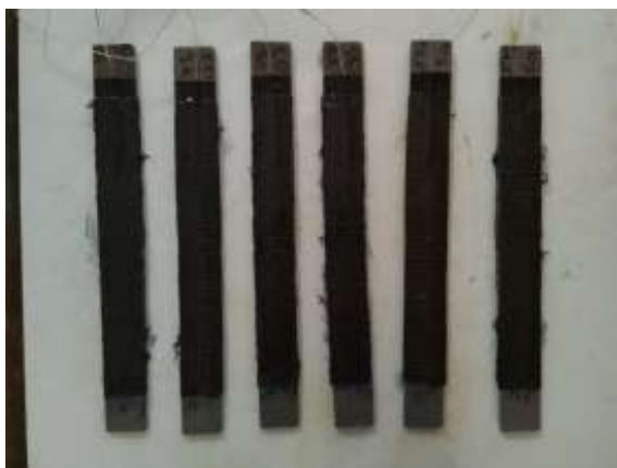
Figure 3.5 Specimen samples after thermos-couple installation
