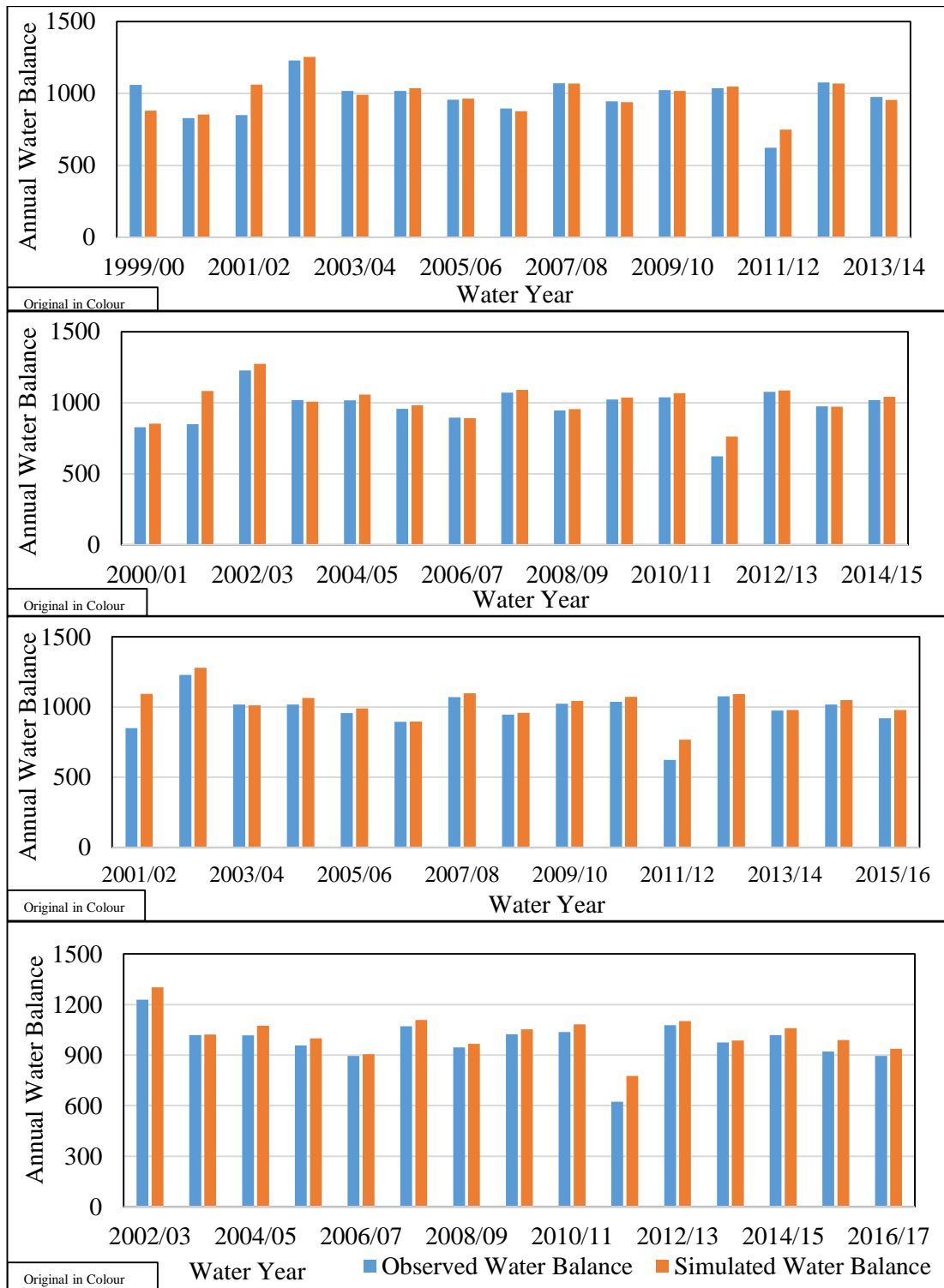
Figure D.206-D.209: Annual Observed and Simulated Water Balance Comparison - 15 year Datasets – Calibration
