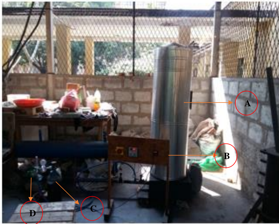
Figure 11 Overall Arrangement A- Combustor, B - Temperature Display, C - CO2 Cylinder, D - Air blower
