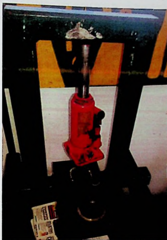
Figure 3.4 Coco peat pellet pressing jig
