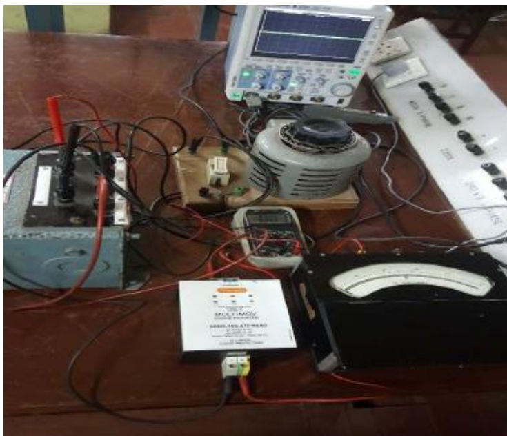
Figure 20: 475V MOV arrester testing
