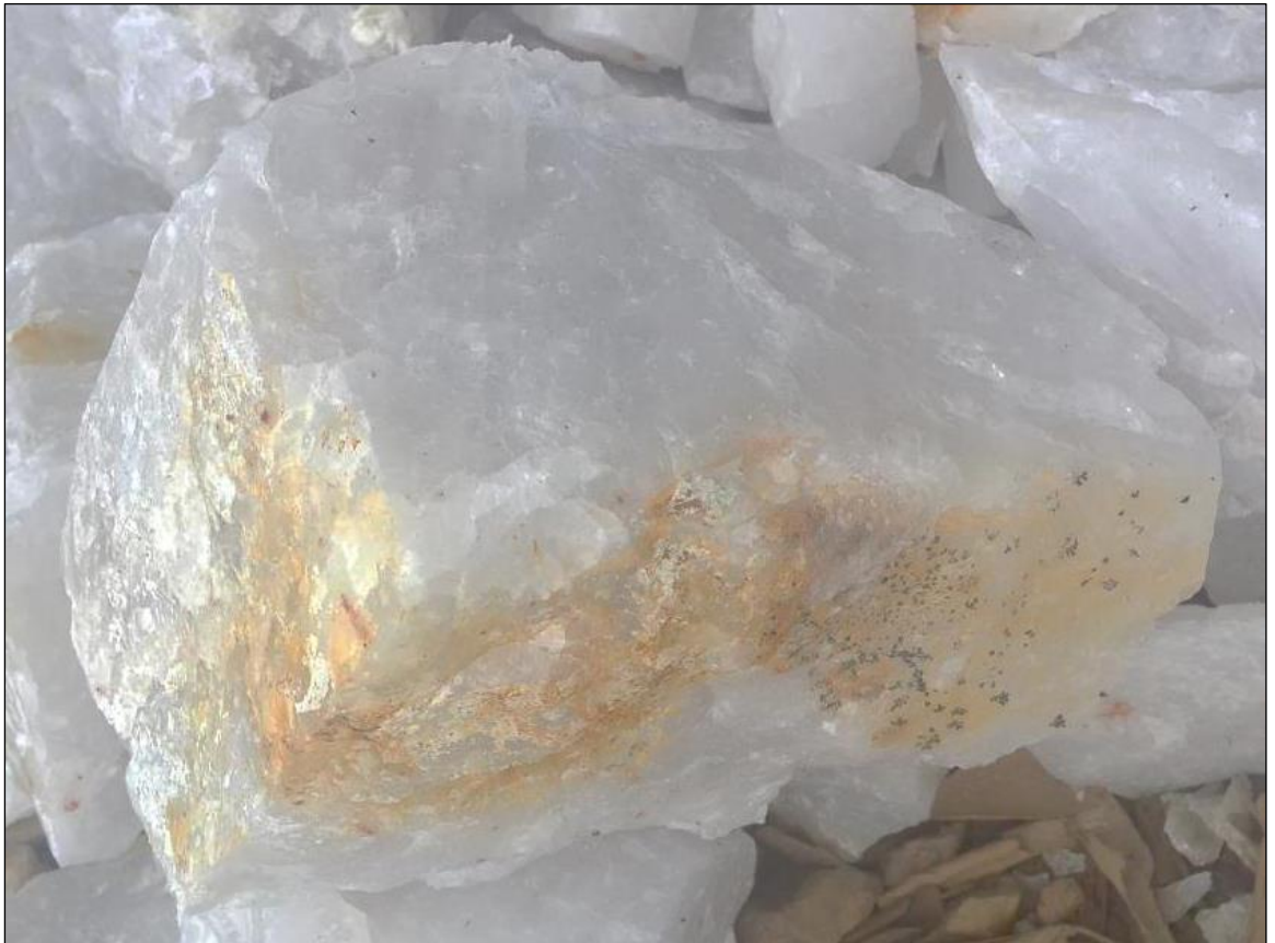
Figure 4.4: Fe stains in milky quartz in selected vein quartz deposits of Badulla
