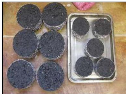
Figure 3: Cored samples used for different tests
