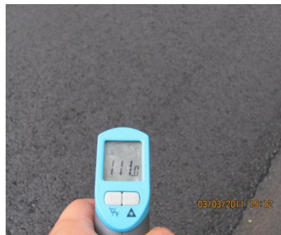
Temperature measurement for WMA-A
