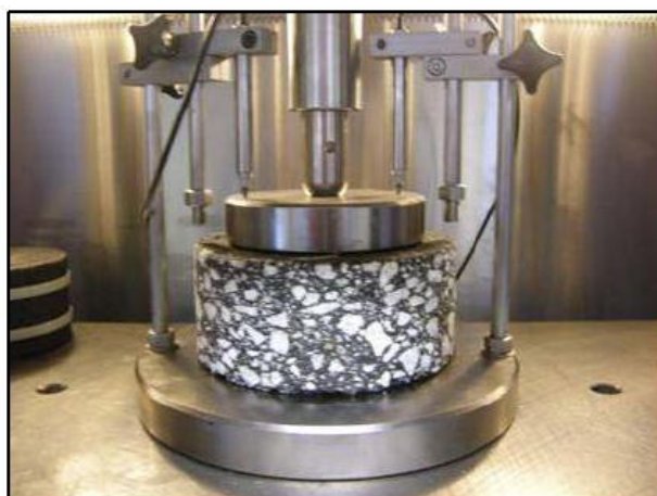
Figure 7: Typical dynamic creep test
