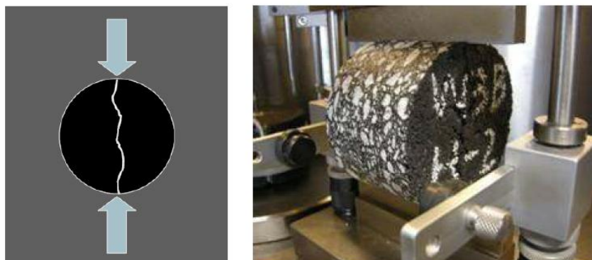
Figure 5: Typical indirect tensile strength test
