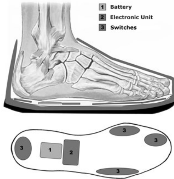
Figure 2.19: ACHILLE interface used to control prostheses. The sensitive areas are marked in the figure [50]. This device contains 4 sensitive areas and can be worn inside a shoe.
