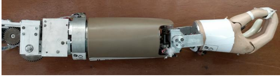
Figure 3.12: Trans-humeral prosthetic arm. The prosthetic arm has 5 DOF: elbow FE, forearm SP, wrist FE, wrist URD, and compound motion of hand. Fabricated prosthesis weighs 3.2kg.
