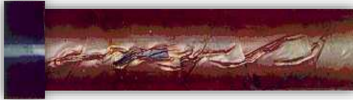
Figure 3-2: Damaged Copper Screen
