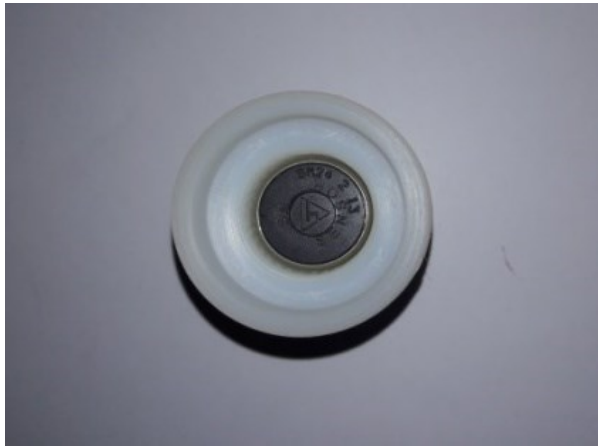
Figure 3.22 Sensor container with geo sensor
