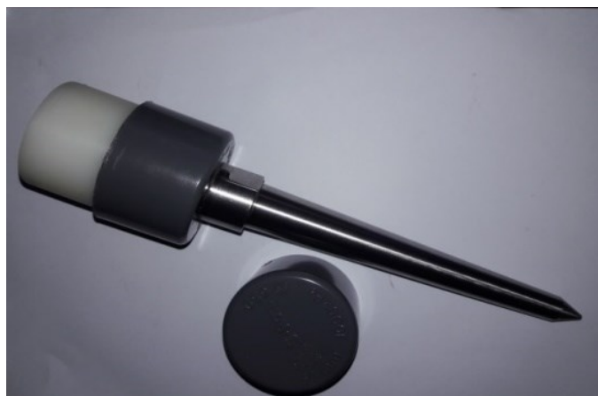
Figure 3.24 Steel Spike & Sensor Container
