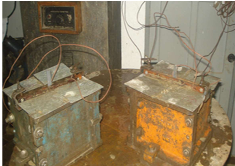
Figure 5-5: Concrete Specimens Out Side the Hot Water Bath
