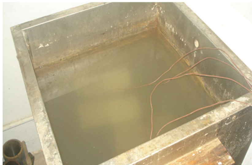
Figure 5-3: Specimens are inside Hot Water Bath
