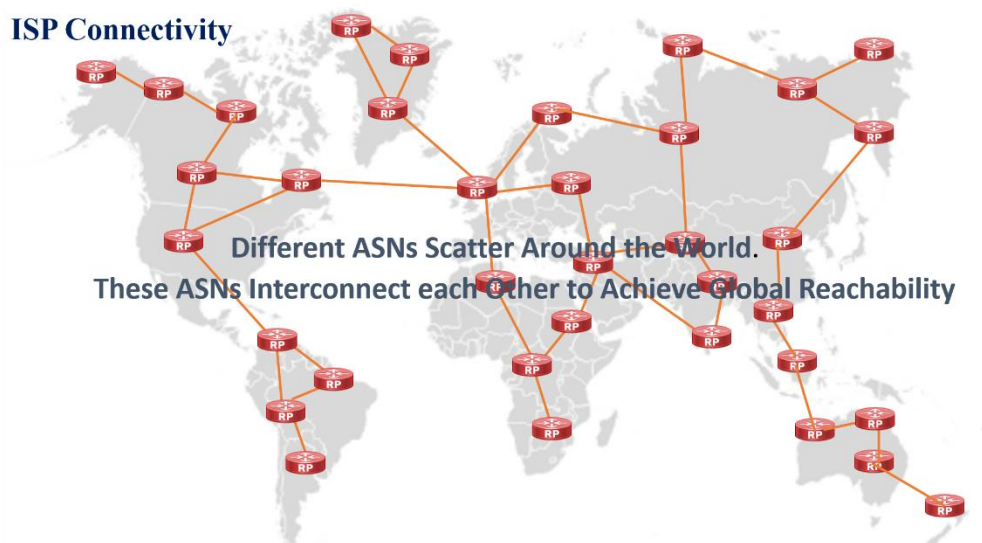
Figure 3: Typical ASN interconnect Scenario
