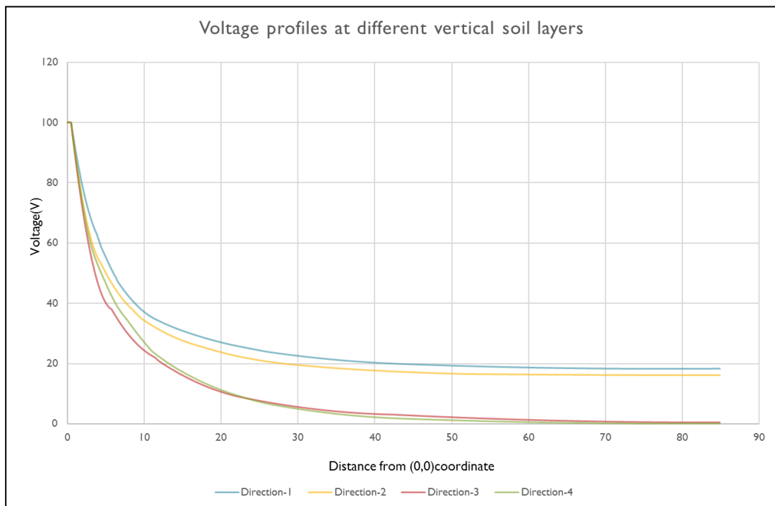
Figure 6.14 directional voltage profiles of each quadrant
