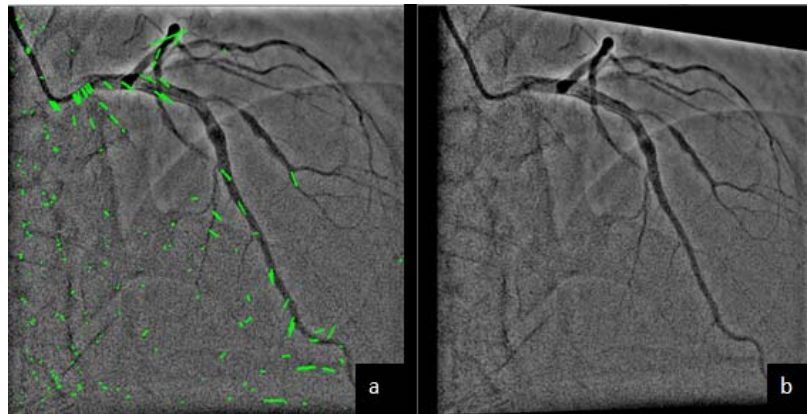
Figure 7.3: Effect of optical flow.
