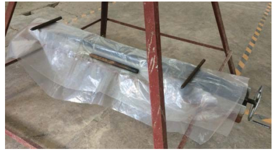
Figure 3.9 Method 2 - Sample kept in the mould undisturbed
