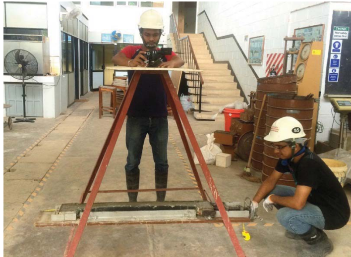
Figure 3.12 Taking photographs from top while applying strain
