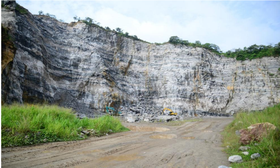
Figure 7.7: View of Single high bench in the operating face of quarry no 07
