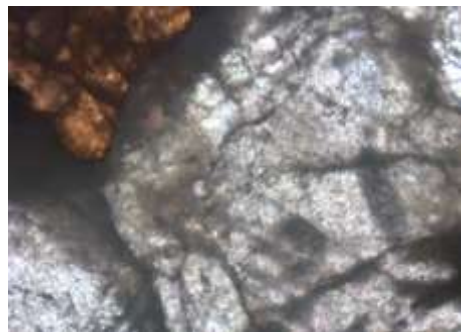
Figure 15 - Microscopic view of the thin section prepared from (450W×6mins) heated in Microwave and quenched rock sample (Magnification : 10X)
