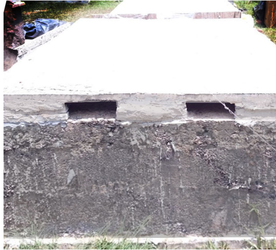
Figure 6.1: The Physical Model Used to Test Air Gap as an Insulator
