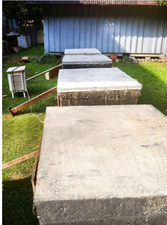
Figure 5.5: Experimental Setup of the Small Scale Physical Models to Compare Thermal Performances
