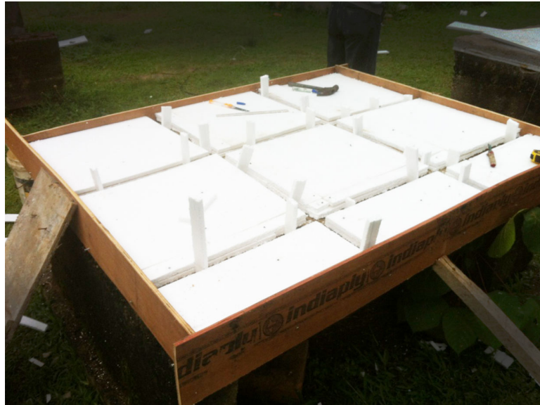
Figure 5.6: Experimental Setup of the System with Continuous Supporting Strips to Compare Thermal Performance
