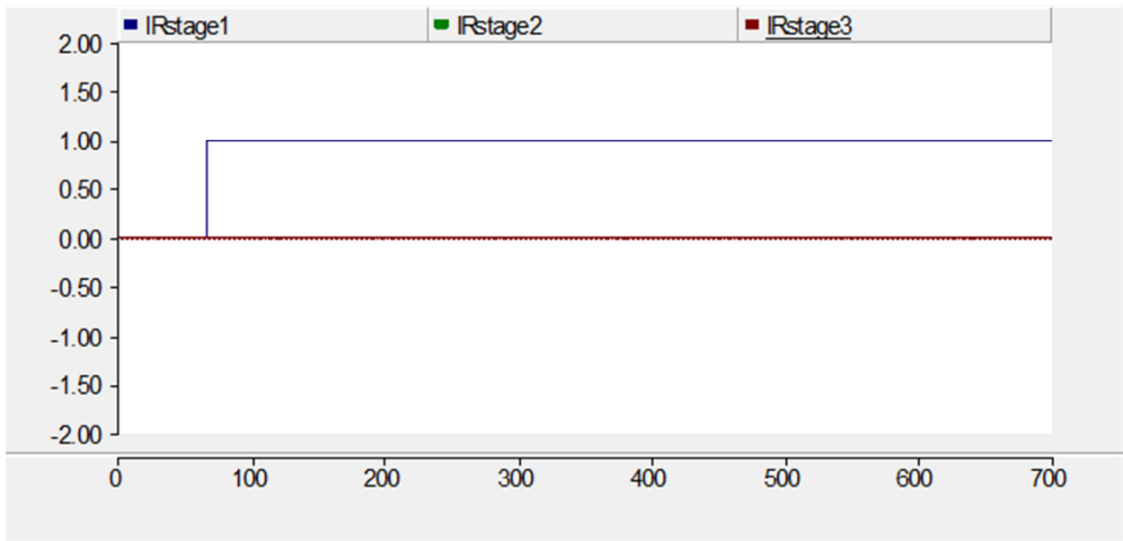
Figure 5:16: 'stage 1' of the load shedding scheme of the Island Rantembe, known as 'IRstage1' got implemented to stabilize the system.
