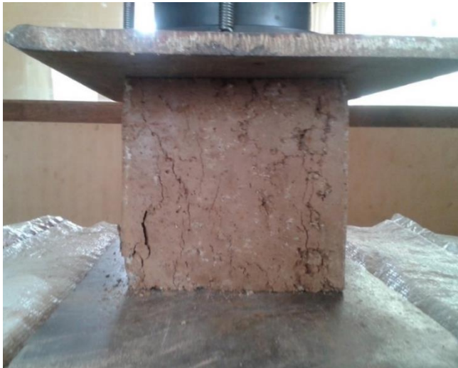
Figure 4 - Testing cubes for compression strength
