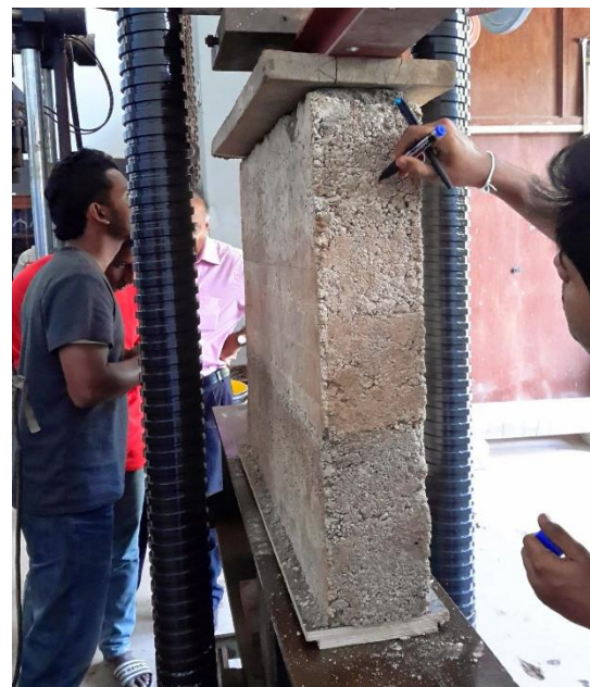
Figure 7 - A panel testing for compressive Strength
