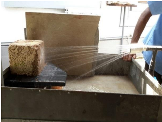
Figure 15 - Accelerated erosion test
