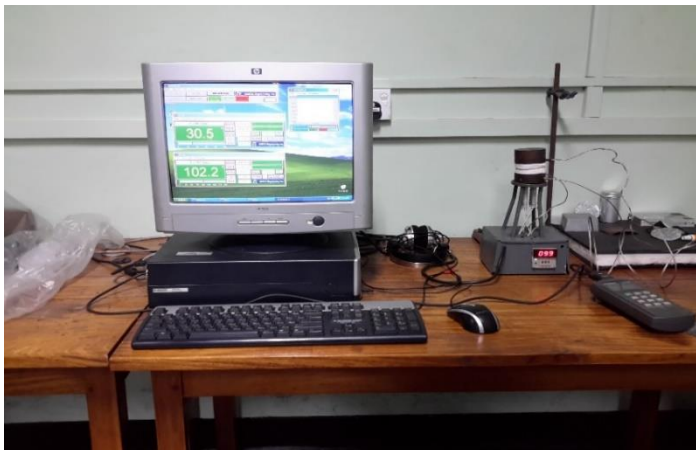
Figure 13 - Thermal Conductivity Testing
