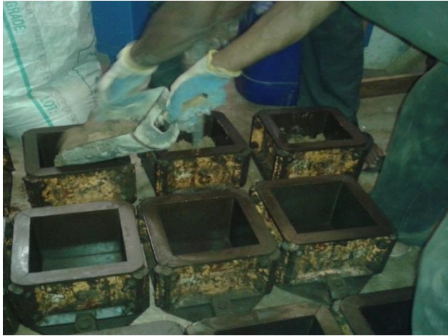
Figure 3 - Casting of test cubes
