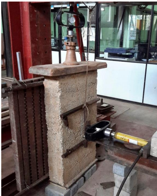
Figure 6 - A panel testing for flexural strength
