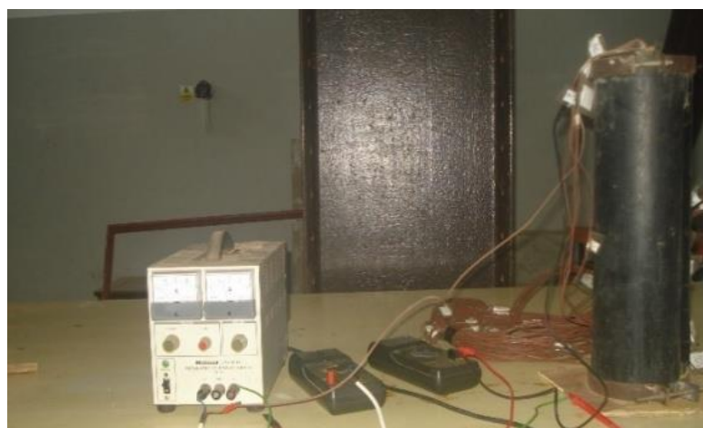
Figure 3-8 : Hot wire testing arrangement
