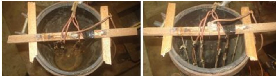
Figure 3-6 : Thermocouples are arranged at required depth and distances
