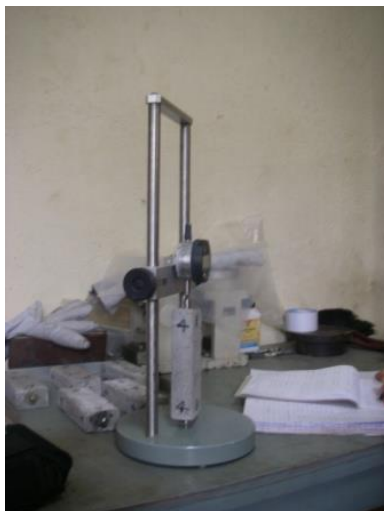
Figure 3-11: Length comparator to measure change in length
