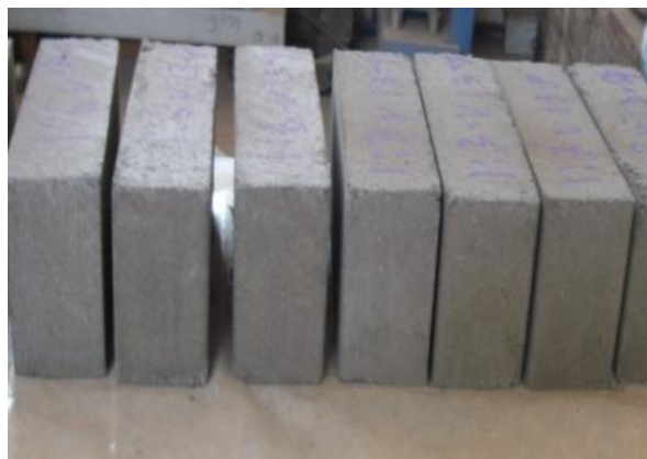
Figure 4-8: Cement-Bottom ash block produced with Cinva-Ram machine
