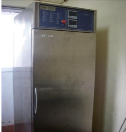
Figure 3-9: Humidity Cabinet to maintain 17% humidity at 50°C
